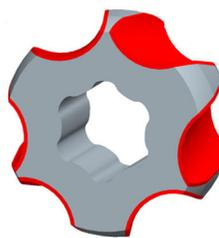
**Fig. 5:** Complex cycloid TO2 profile ( $n=6$ ,  $e=0.15$ )
