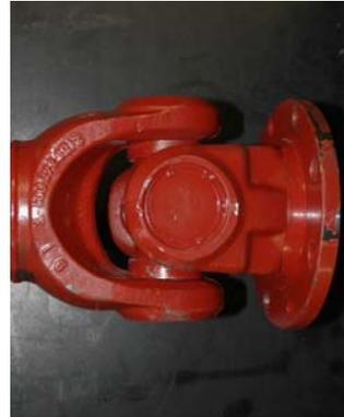
*Due to the installation situation, cardan shafts can be used to transmit the power between motor drive and gear box. To verify the real stresses and strains, torque and bending moment as well as axial forces are measured. With these results design and dimensioning of the power train can be enhanced.*
