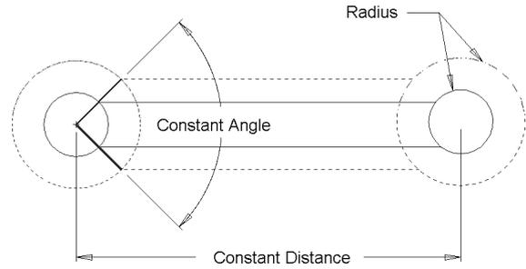
**Fig. 8** Bore Radius representation with constant distance.
