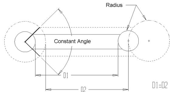
**Fig. 9** Bore Radius representation with constant length.
