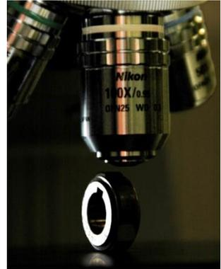
*A new laser-scanning-microscope enables students and scientific staff to examine technical surfaces. Besides high-resolution true-color images height information is detected, which allows to generate 3D-surface-models.*
