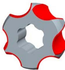
**Fig. 5:** Complex cycloid TO2 profile (n=6, e=0.15 )
