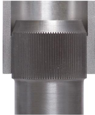
*The following article is presenting a summary of the parameters that are influencing the joining process of knurled shaft-hub-connections. In addition to the influence of joining length, hub wall thickness and material combination, the joining process of thin-walled hubs in knurled shaft-hub-connections is discussed on the basis of current investigation results.*
