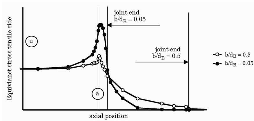
**Figure 4. Comparison of stress distribution over the splined joint width in the shaft tooth root for various ratios of width to diameter  $b/d_B$**
