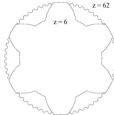
**Figure 2. Comparison of the cross section of splined shafts of the same reference diameter with small and large numbers of teeth**
