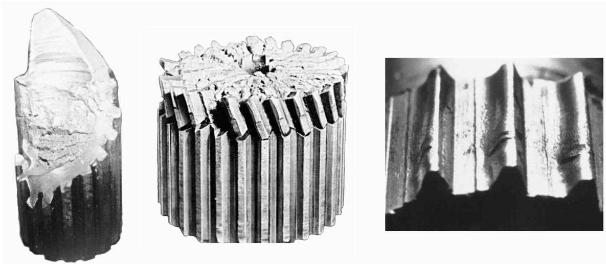
**Figure 1. Damage to involute splines. left: fatigue fracture of a spline, middle: brittle fracture, right: appearance of wear**
