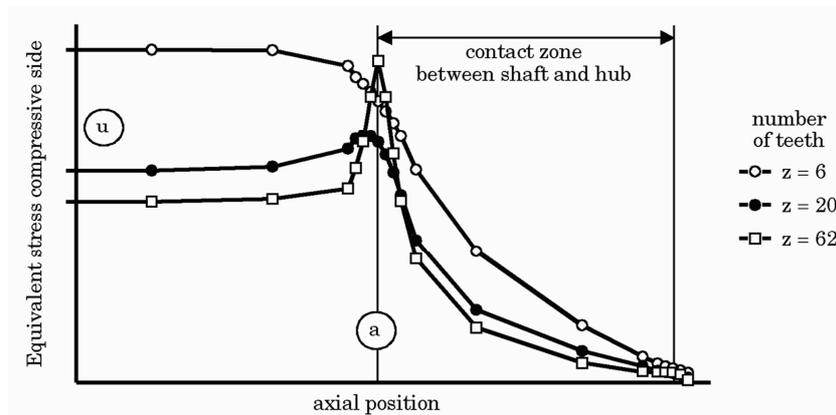
**Figure 3. Comparison of the distribution of stress at the spline root over the splined joint width for different numbers of teeth**
