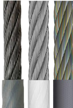
*For coated ropes exists no discard criteria referring to current standards. In some practical cases coated ropes show a longer service life than wire ropes. Experiments on bending fatigue and spooling behaviour are carried out to utilise this advantage and optimise the coating. The research project is supported by the Drahtseil-Vereinigung e.V. and is carried out by the TU Dresden and the TU Clausthal.*
