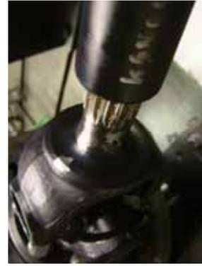
*Cardan shafts are used in many different applications with varying loads. The two cardan joints and especially the splined length compensation are critical elements under both, torsional and bending loads. To determine the life time of such a splined length compensation, the IMW makes experimental and numerical investigations.*
